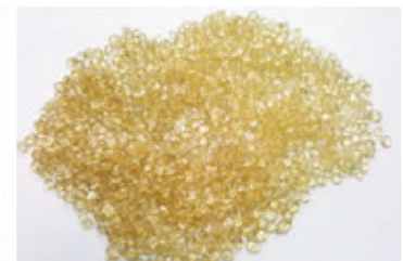
Polyphenylsulfone (PPSU), a plastic used as raw material in nursing bottles
